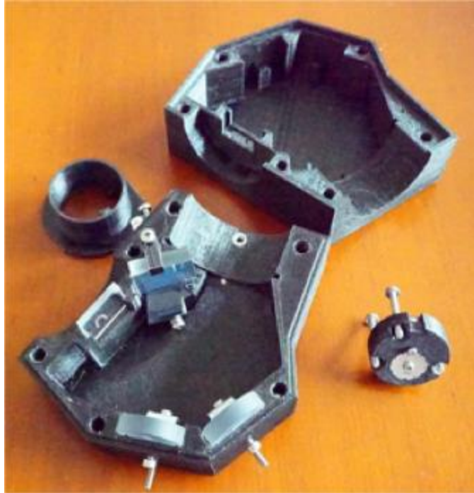
Figure 4 – An early UVEX 3D printed Prototype
