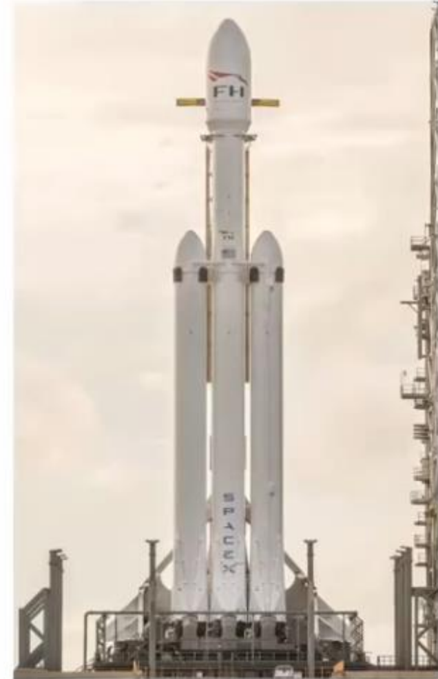
One fully-fueled Falcon Heavy (both stages) \sim 156 mT RP-1, \sim 43 MJ/kg = \sim 6.7 \times 10^6 MJ
