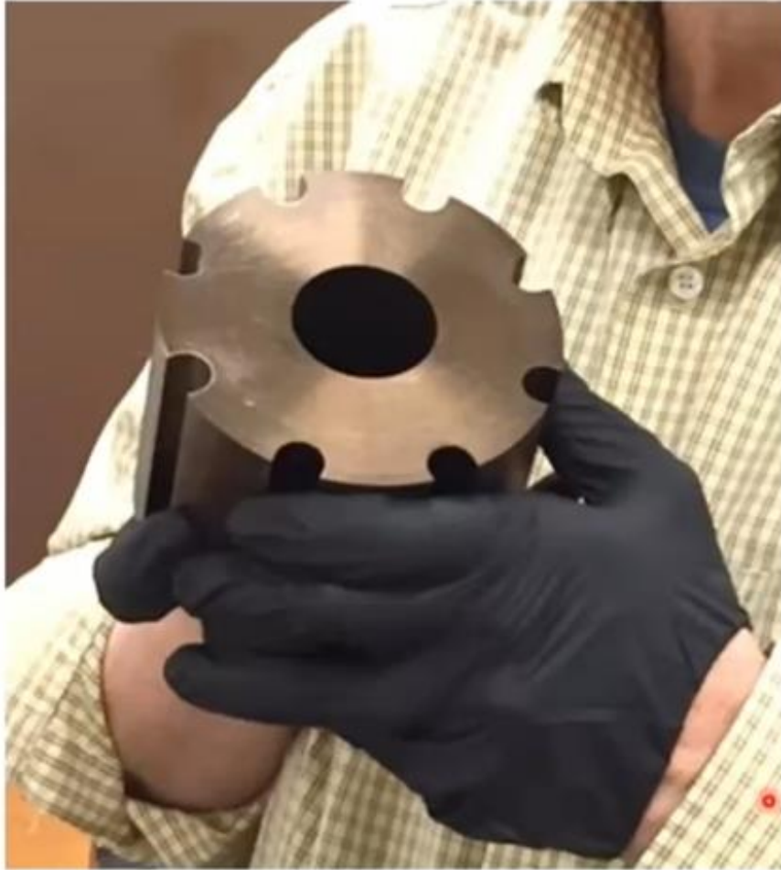
One KRUSTY Piece = 10.7 kg U8Mo This piece = \sim 8.1 \times 10^8 MJ if all U atoms are burned
